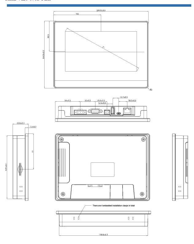
Embedded installation hole size: 192 \* 138 (+ 1.5mm / - 0.0mm)
